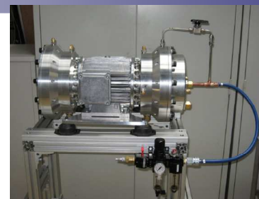
Enefcogen HT scroll turbine and prototype
